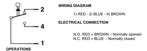
The PR5 Pressure switch signals the surpass of a pre-set pressure, through a piston, which operates a switch lever. The set pressures are respectively; 10 bar - 1 MPa; 15 bar - 1.5 MPa; 25 bar - 2.5 MPa and 40 bar - 4 MPa of the fixed type.
