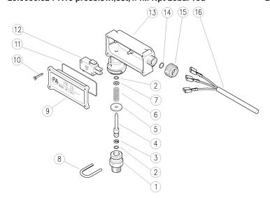
29.0035.62 PR16 press.sw.,sst,3/8M Npt 25bar red 29.0040.00 PR16 press.sw.,brass,3/8M Bsp 40bar blck 29.0040.11 PR16 press.sw.,brass,3/8M Bsp 15bar blue 29.0040.20 PR16 press.sw.,brass,1/4M Bsp 40bar blck 29.0040.30 PR16 press.sw.,brass,1/4M Bsp 25bar red 29.0040.40 PR16 press.sw.,brass,1/4M Bsp 15bar blue
